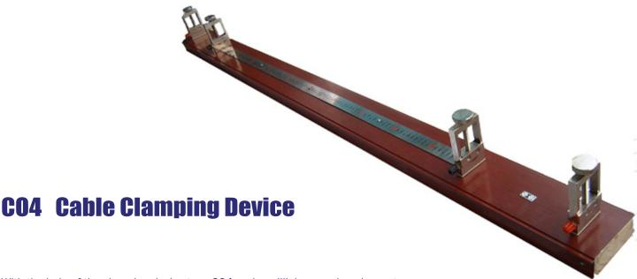
With the help of the clamping device type CO4 and a milliohm or microohmmeter the ohmic resistances of cable samples and materials such as cords and strips can be measured. Fields of application include production monitoring, quality assurance and general test measurements.
